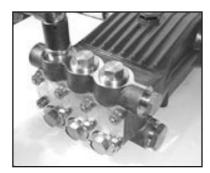
With a 30mm wrench, remove the six (6) plugs (48) from the valve casing (43). Inspect the o-rings (48A) and replace if necessary. Remove the complete valve assembly (46A) by threading a 12mm bolt into the spring retainer and pulling straight out.
